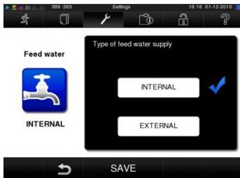
Depending on whether the feed water supply should come from the internal storage tank or you have connected a water-treatment system, select the appropriate setting on the display:
