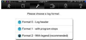
For each completed program, a log is stored in the internal log memory. Via the log format, you can specify which of the stored data should be output. You can choose between a short (0), medium (1) and long form (2).
