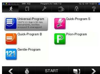
The program-specific drying times ensure a very good drying of →the sterilized items in the case of a loading as described in this chapter (see page 20, **Loading the autoclave**). For difficult drying tasks, you can extend the drying time of a program by 50% in the **Settings** menu via the option **Supplement Drying**.
