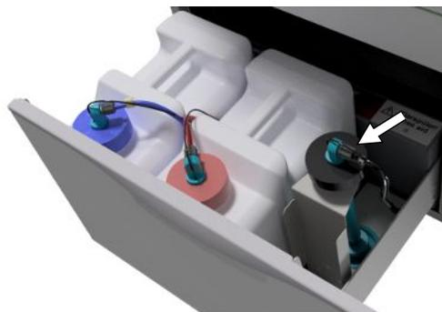
2. The process agent hoses only need to be placed head-first in the suction lance bracket if the metering hoses are to be bled, see [Removing air from the metering system](#) [▶ page 25].
