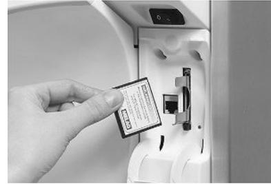
3. Slide the CF card in the card slot until it clicks. Do not use force. When the CF card has been placed correctly, the red LED will illuminate shortly.
