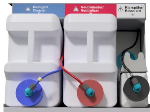
**Replacing the containers for cleaning agent and neutraliser**
